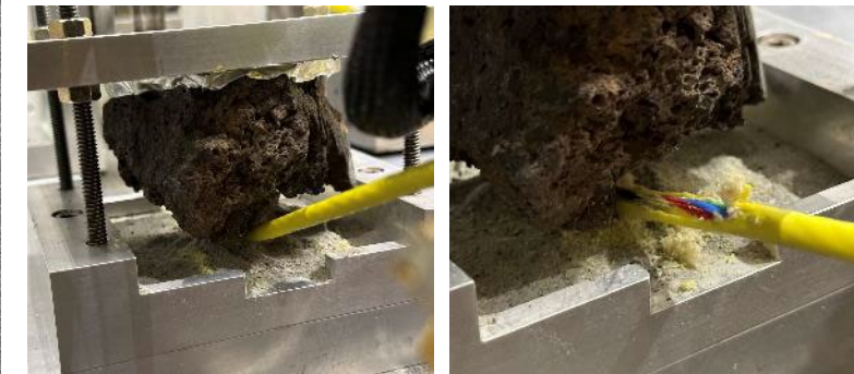
Abrasion testing of tether in Lunar thermal environment
